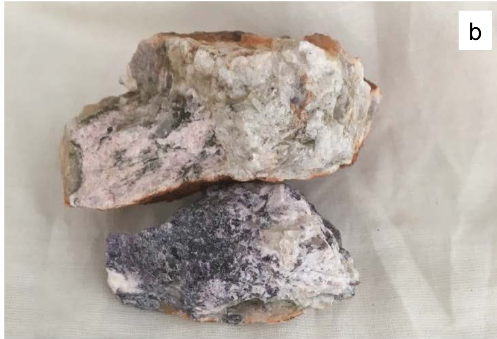
(a) Thin section showing dominant spodumene; (b) Spodumene (top) and lepidolite (bottom) collected from the Marble Bar Lithium Project E45/4669
